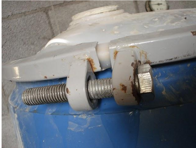
Buckling of one the BYOW System's lid and water leakage – Nov 2008
